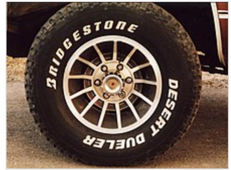
W. R. Grace & Co. 13 spoke 15"x8.5" aluminum wheel, OEM, 1978 Chevrolet K5 Blazer Cheyenne
